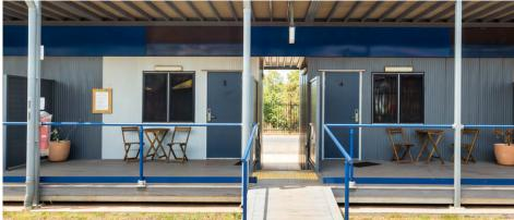
This custom-designed two-storey turnkey modular hotel building was designed and manufactured in Brisbane and transported via road and barge to Bamaga on the northern peninsula of Queensland for installation.
